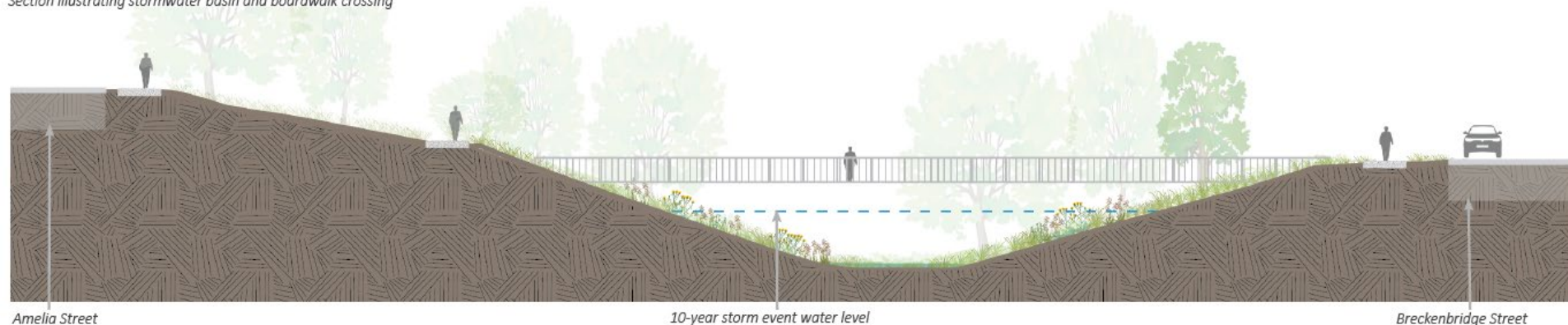
Section illustrating stormwater basin and boardwalk crossing
